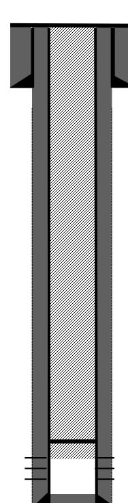
7" 20# J-55 casing @ 127' Hole size 9-1/8" Cemented w/ 59 Cu.ft Class B. Circ 2 bbls cement to surface
