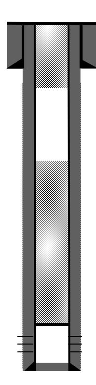
7" 23#, J-55 casing @ 120': Hole size -9-1/8" Cemented with 80 sks, Class B cement. Circulate cement
