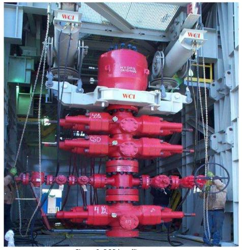
Figure 3. BOP handling system
