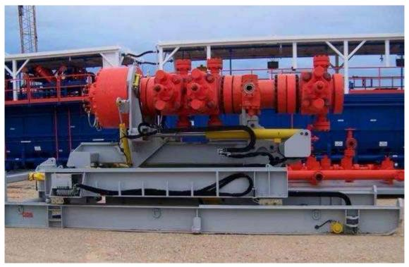
Figure 4. BOP handling system
