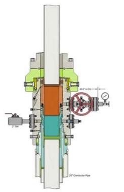
Run 7 5/8" Casing Land Casing on 7 5/8" Mandrel Hanger Cement 7 5/8" Casing Retrieve Running Tool
