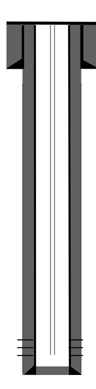
5-1/2" 14#, 8rd casing @ 32': Hole size - 7-7/8" Cemented with 5 sks.
