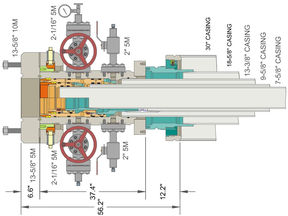
30" X 18-5/8" X 13-3/8" X 9-5/8" X 7-5/8" 5M RSH-2N WELLHEAD ASSEMBLY,
