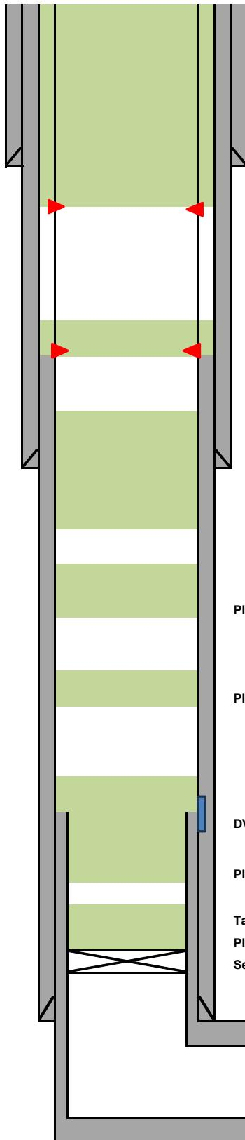
Plug (# 8) Rigged up pump and circulated (180 sxs) class (c) cement from (450) to surface.
