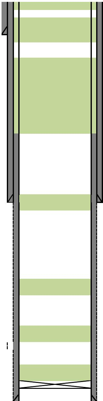
Plug (# 7) Rigged up pump and circulated (35 sxs) class (C) cement from (100) to surface.
