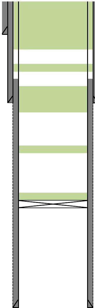
Plug (# 6) Spot (15 sxs) class (c) cement From (60) to (surface).
