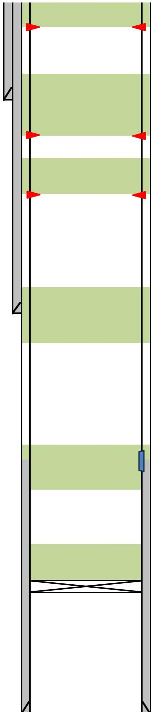
Plug (# 6) Rigged up pump and circulated (40 sxs) class (C) cement from (100) to surface.
