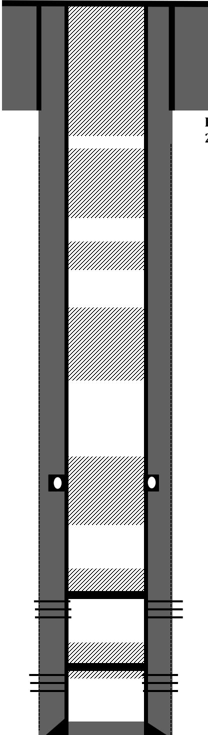
8-5/8" J-55 24# casing @ 204'. Cemented with 135 sks, 159 Cu.ft Cement.
