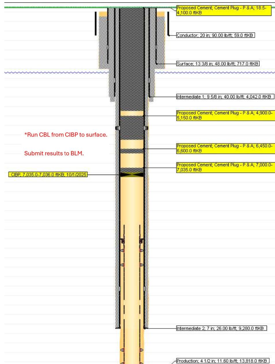
Spot Class C cement from 4,100' to surface.
