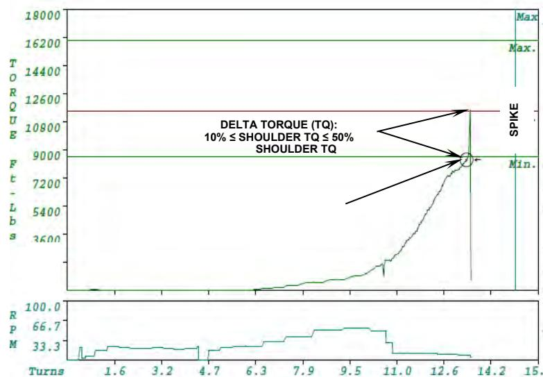
Similarly, random connections here and there with more than 50% **Delta Torque** is generally not cause for concern. However, if overshooting the 50% maximum **Delta Torque** target occurs frequently, then the established **Running Torque** value should be walked down in 500 ft-lbs. to 1,000 ft-lbs. increments until connection makeup routinely falls in line with the stated acceptance criteria.
