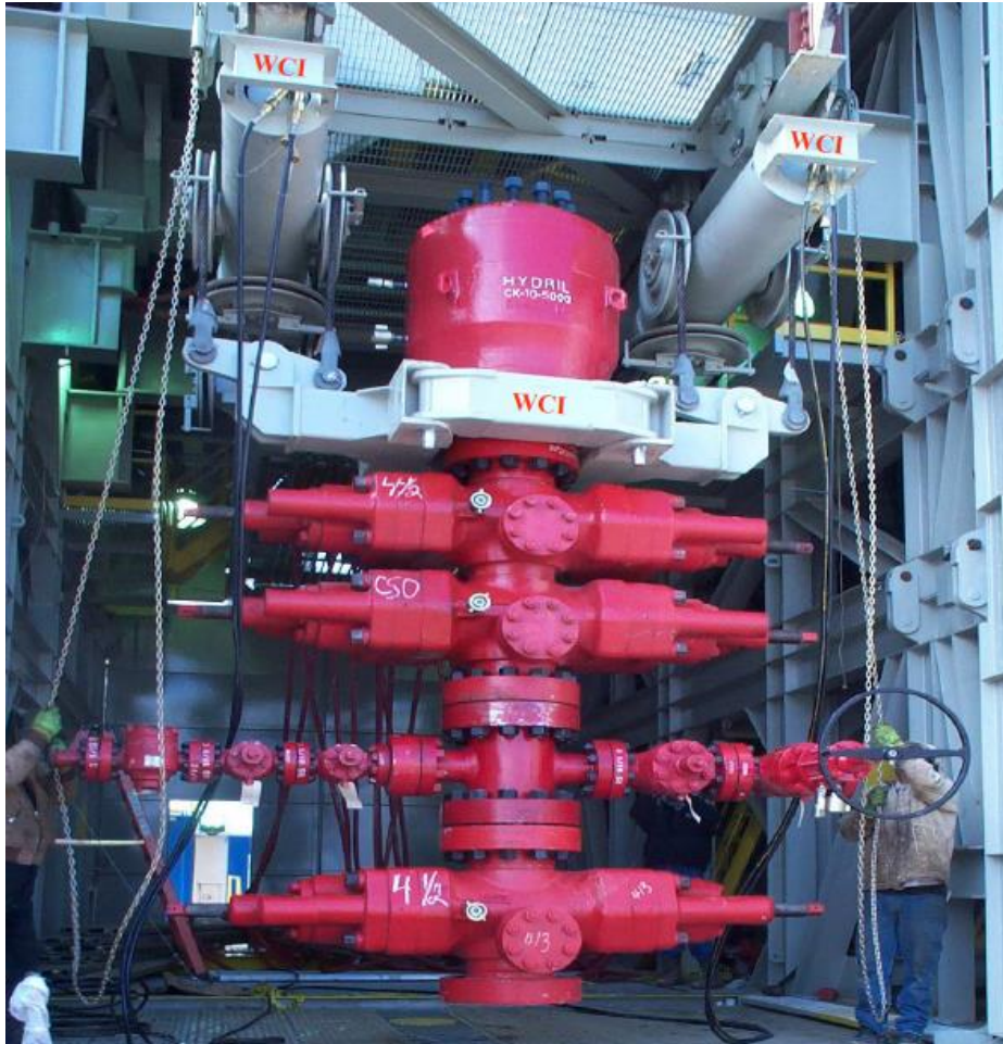
Figure 3. BOP handling system
