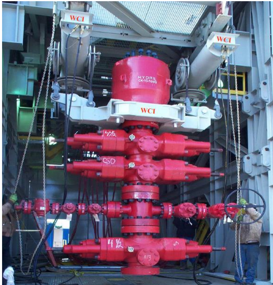
Figure 3. BOP handling system
