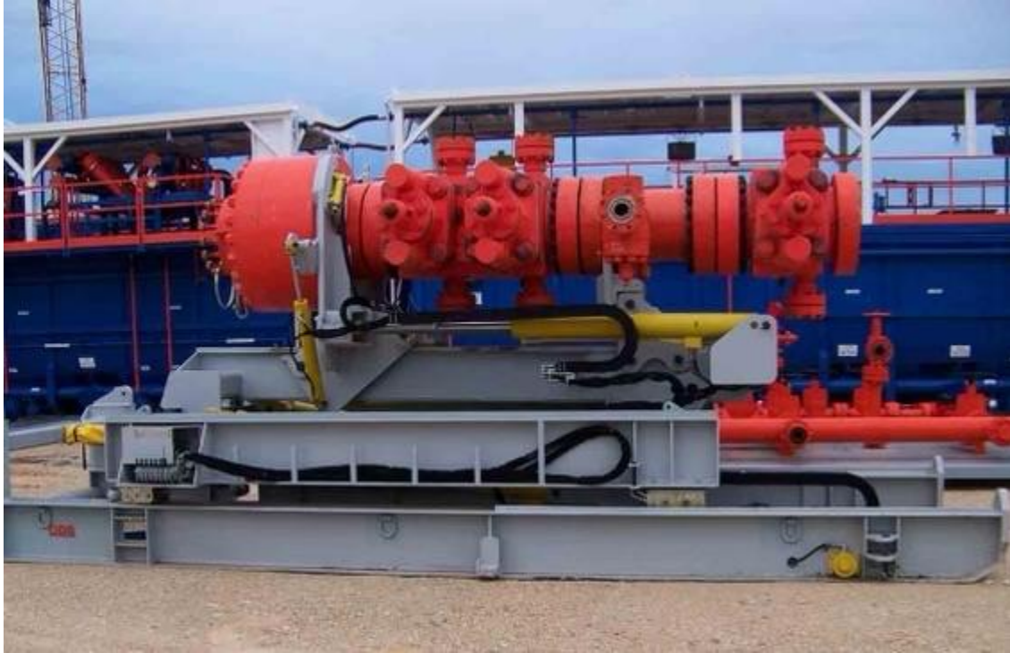
Figure 4. BOP handling system
