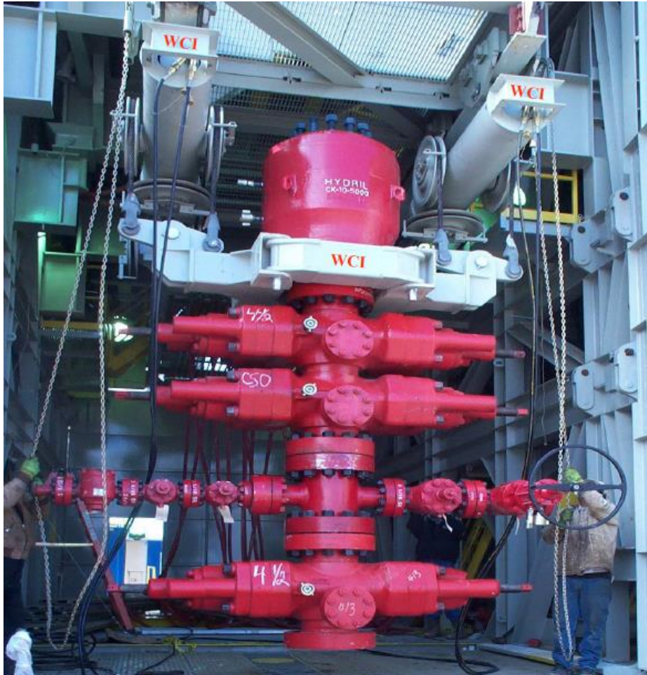
Figure 3. BOP handling system
