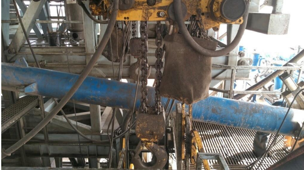
Figure 2: BOP Winch System
