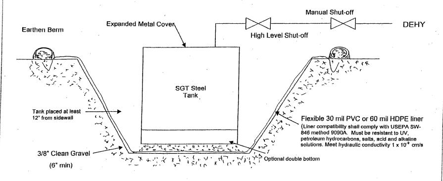
Note: Foundation shall be free of rocks and debris and otherwise made level. Liner is anchored at ground surface - min 12 in trench. Installation allows for fluid collection point and visible inspection of exposed liner. Shut-off system designed to maintain 28" freeboard. Installation location should meet siting criteria or be approved by NMOCD.
