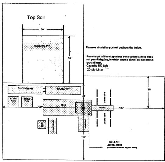
Cellar can be 4X4X4 if using a screw-on wellhead
