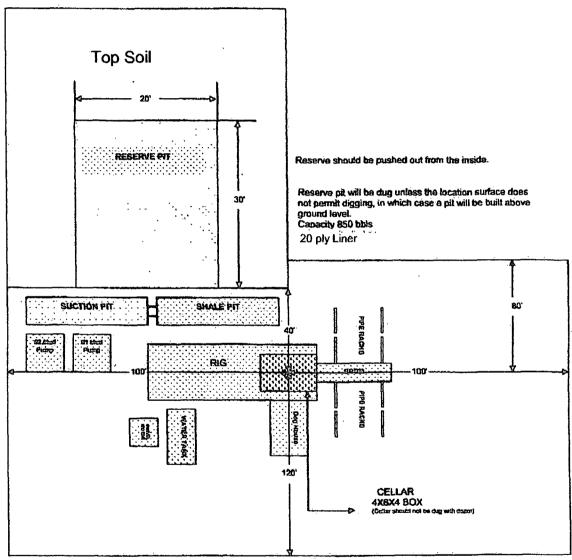
Cellar can be 4X4X4 if using a screw-on wellhoad
