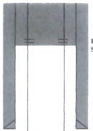
Perforate 5 1/2" csg. @ 350'. Squeeze cmt. to surface w/175 ss.
