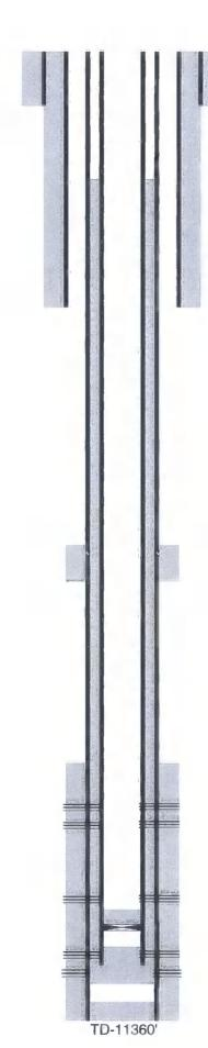
17-1/2" hole @ 615' 13-3/8" csg @ 615' w/ 895sx-TOC-Surf-Circ
