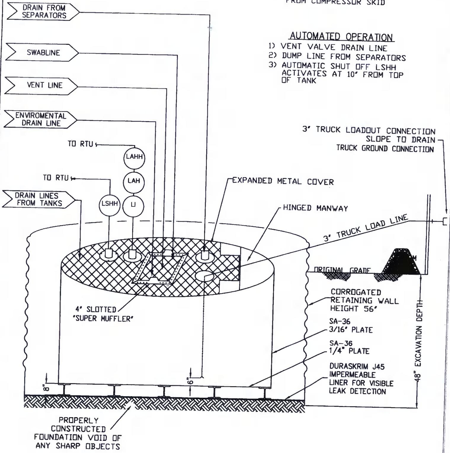
3" TRUCK LOADOUT CONNECTION
