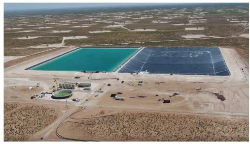
Image: Longfellow's 2MMBbl Produced Water Recycling & Storage Facility
