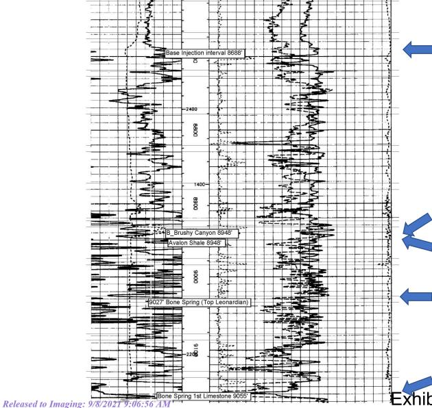
**Base of DMG Injection zone 5267' – 8688'** Limestone, interbedded Shale and Siltstone
