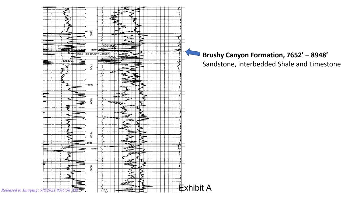
Exhibit 4: Base Brushy Canyon Formation, Top Avalon Shale, and Bone Spring Formation 30-025-35322 Gamma Ray, Caliper, Density - Neutron Porosity Log
