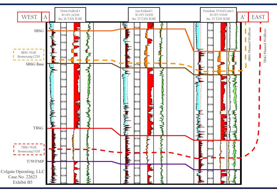
Stratigraphic Cross Section A-A' (SBSG and TBSG) Boomerang 25 Fed Com
