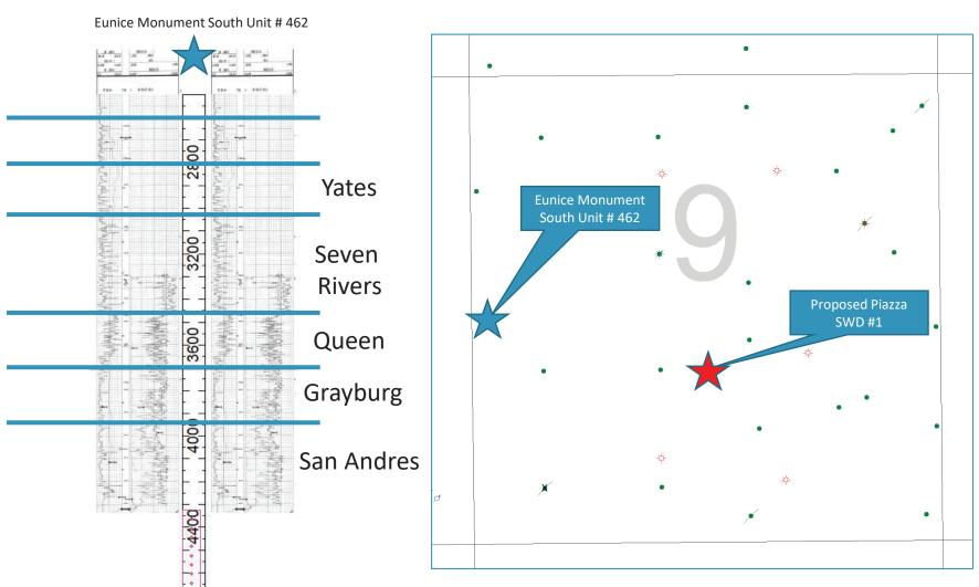
The Goodnight Midstream, Piazza SWD #1 is proposed as marked on the map above. The application states that the injection disposal interval will be within the San Andres formation between approximately 4,125' and 5,400' TVD.
