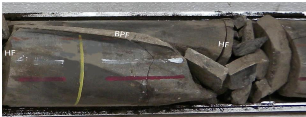
Fig 55—Bed-parallel natural fracture (BPF) filled with fibrous calcite (beef) is parted along both faces. The fractures bounding the section with parted beef are hydraulic fractures (HF). Our interpretation is that the hydraulic fracture caused reactivation of the natural fracture. Core 8.
