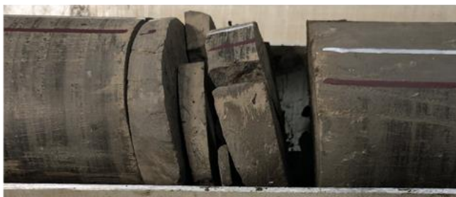
Fig 54—(a) Four-fracture swarm in Core 2. The four HFs are the leftmost fractures, the two on the right (uphole) are interpreted as drilling induced. This swarm contained some fine sand patches (see Fig 61). (b) Five-fracture swarm in Core 6.
