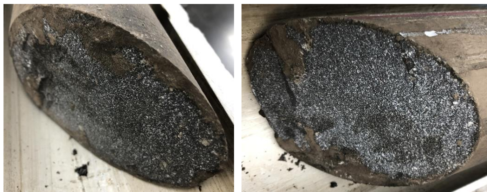
Fig 56—Drusy calcite cement on both the uphole (left) and downhole (right) faces of a Set 1 fracture in Core 9. Interpretation is that this fracture was possibly open in the subsurface. The reason for fracture reactivation in this case is likely core handling.
