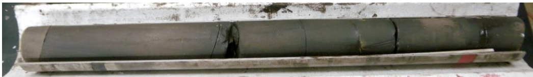
Fig 53—Hydraulic fracture doublets in three tubes from Core 3: (a) in middle of tube, (b) above the yellow foot marker, (c) center left of tube.
