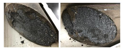
Fig 56—Drusy calcite cement on both the uphole (left) and downhole (right) faces of a Set 1 fracture in Core 9. Interpretation is that this fracture was possibly open in the subsurface. The reason for fracture reactivation in this case is likely core handling.
