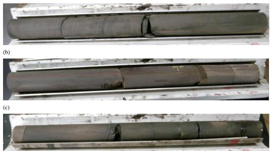
Fig 53—Hydraulic fracture doublets in three tubes from Core 3: (a) in middle of tube, (b) above the yellow foot marker), (c) center left of tube.
