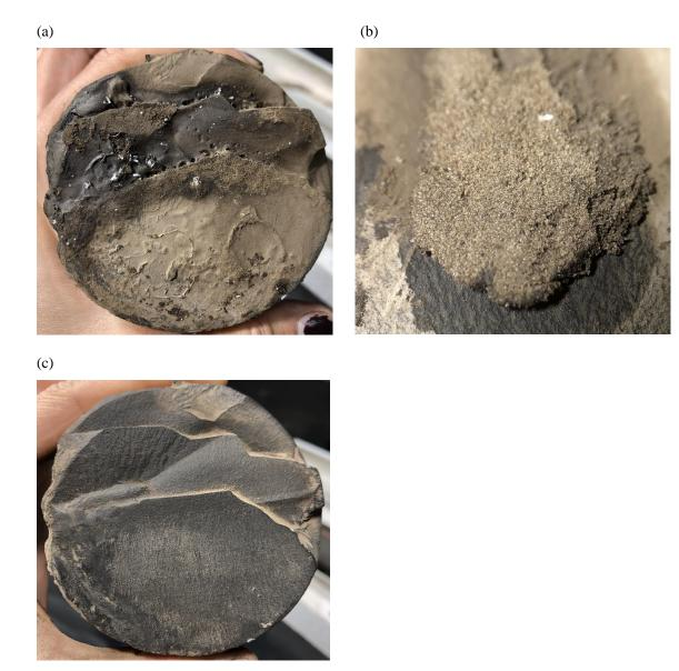
Fig 61—(a) fracture face showing sand patches (b) close-up of patch, field of view  $\sim$ 1 cm. (c) cleaned face showing steps and twist hackles.
