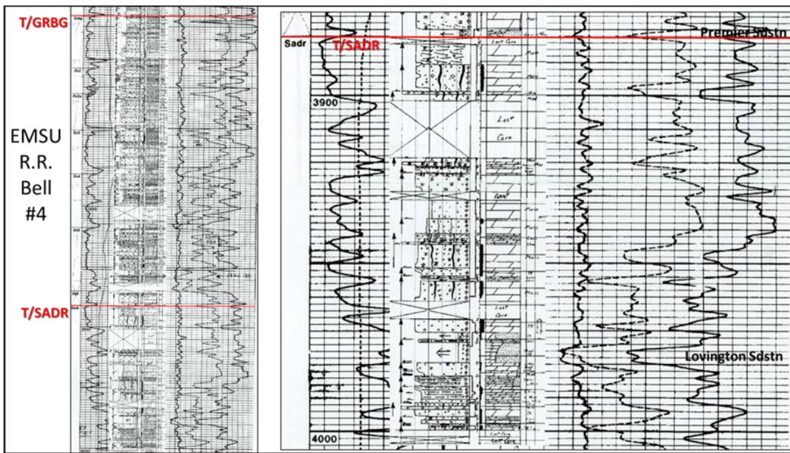
Figure B18. Left is R.R. Bell #4 well log and core description of the complete Grayburg reservoir and San Andres reservoir residual oil zone (ROZ). Right is a close-up view from Premier Sandstone and unconformity (red line) that separates overlying Grayburg reservoir from underlying San Andres reservoir residual oil zone (ROZ). San Andres core penetrated to beneath the Lovington Sandstone.
