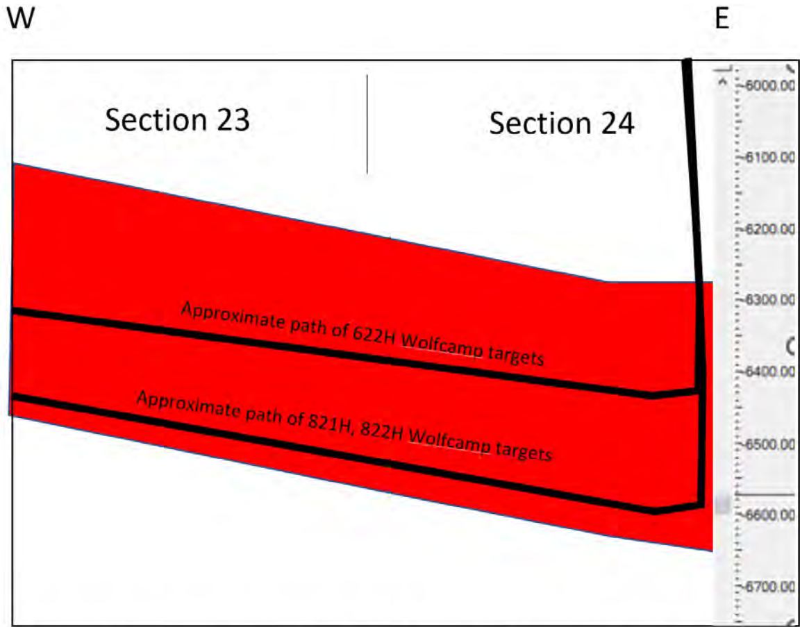
Exhibit B-6 is a cross section with approximate well trajectory
