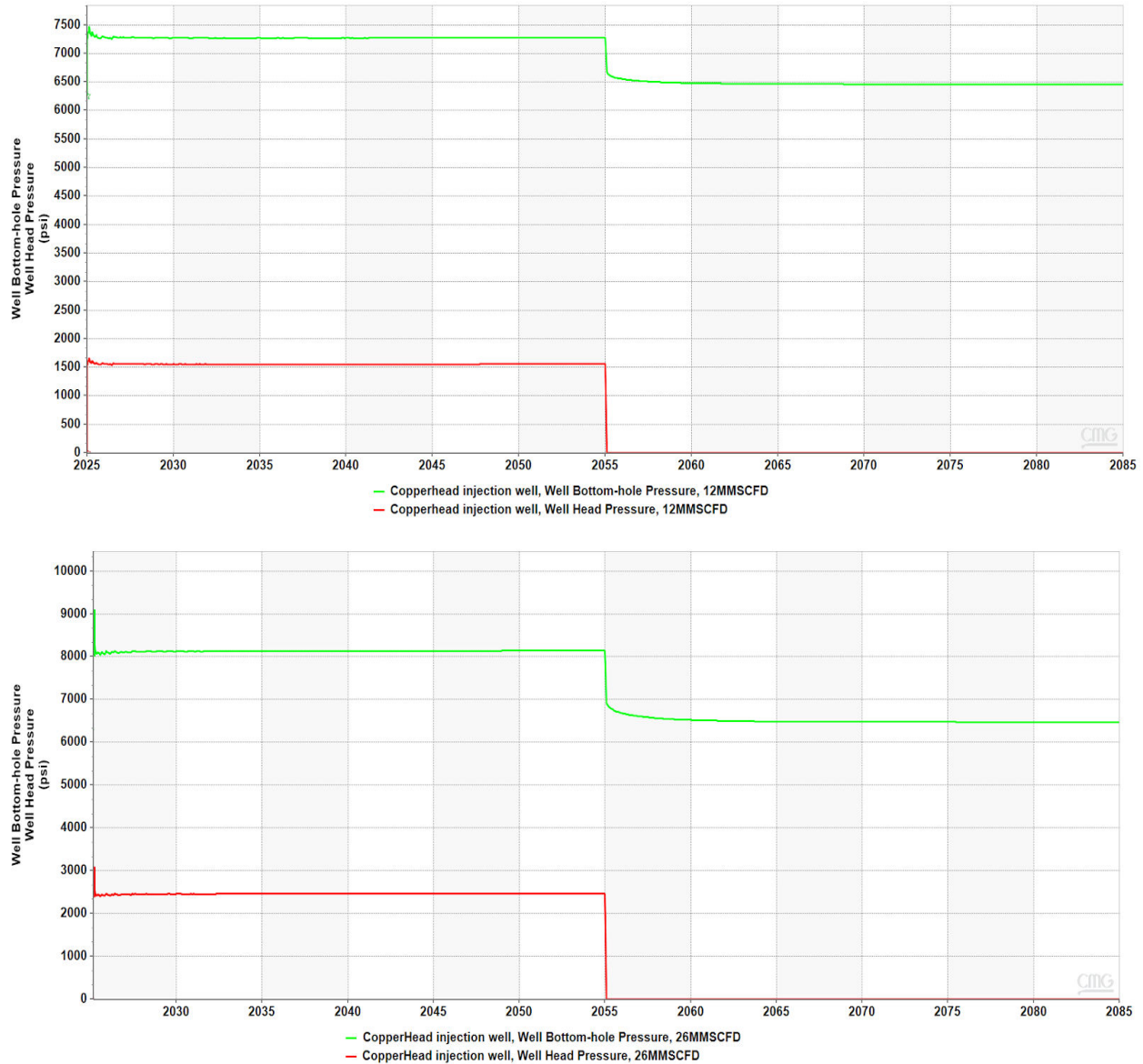
Figure IV-6 Bottom hole pressure (red) and wellhead pressure (green) of Copperhead AGI #001 at 12 MMSCFD (top) and 26 MMSCFD (bottom)
