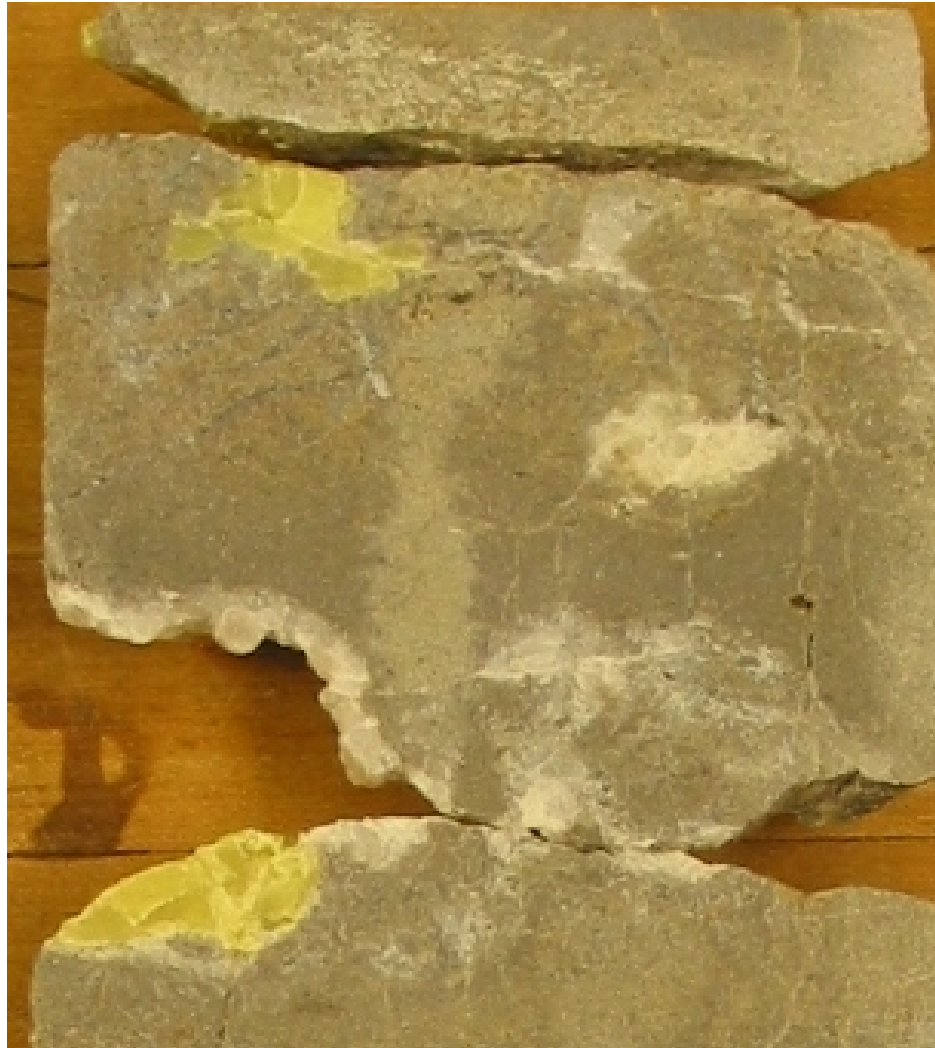
Core with native sulfur and calcite filling voids from interval below the main pay in the lower San Andres in McCamey Field.
