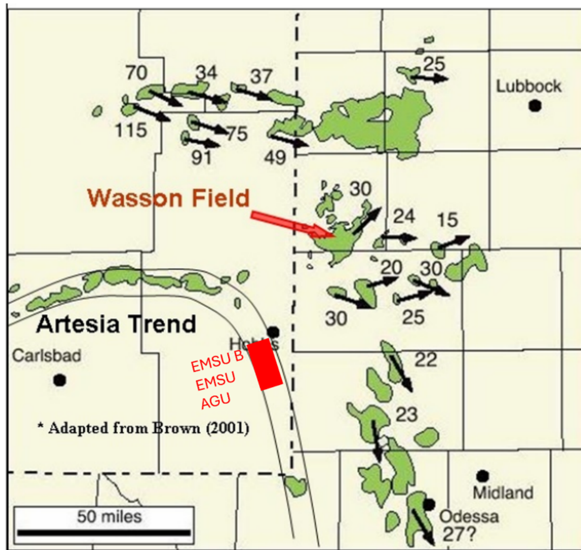
Distribution of tilted oil/water contacts in the Northwest Shelf and Central Basin Platform areas of the Permian Basin. After Brown, 1999.
