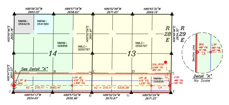
= SURFACE HOLE LOCATION/KICK OFF POINT = FIRST TAKE POINT/LAST TAKE POINT = LEASE PENETRATION POINT = BOTTOM HOLE LOCATION
