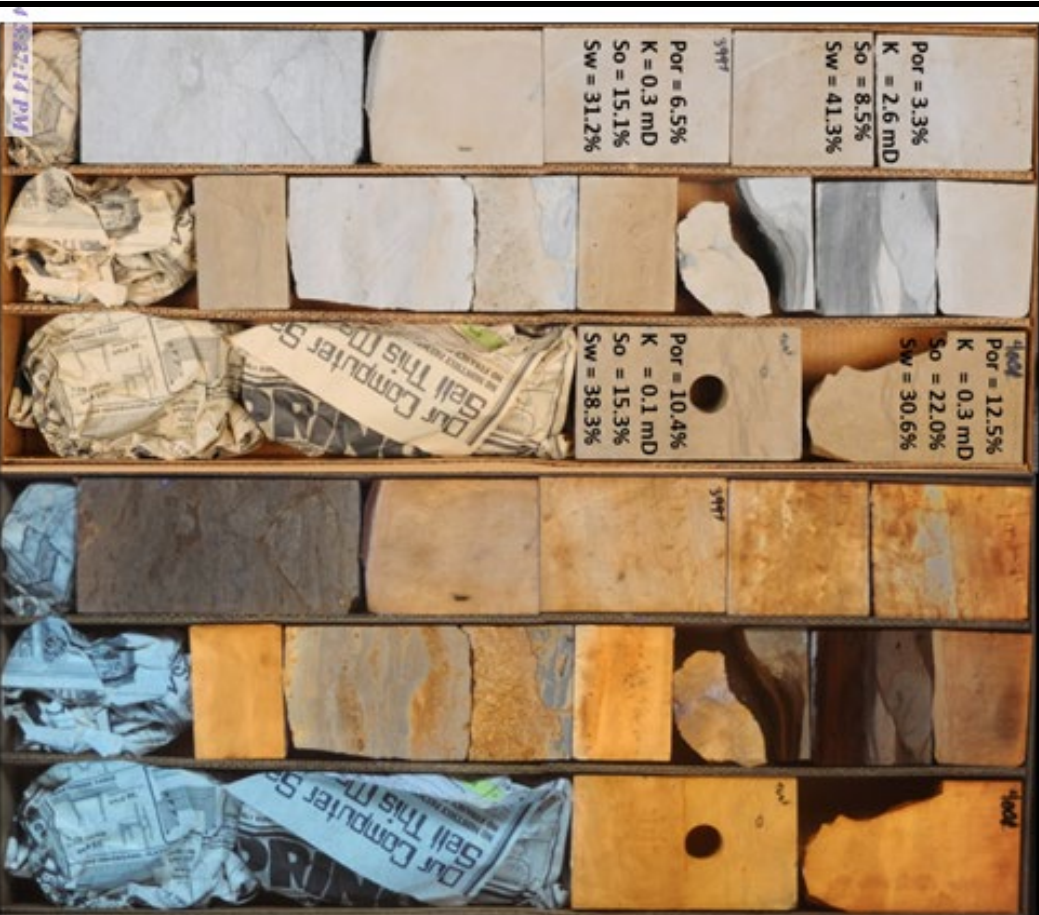
Exhibit L-11: One of the key indicators of an ROZ, the staining of the core with oil over the San Andres is strong
