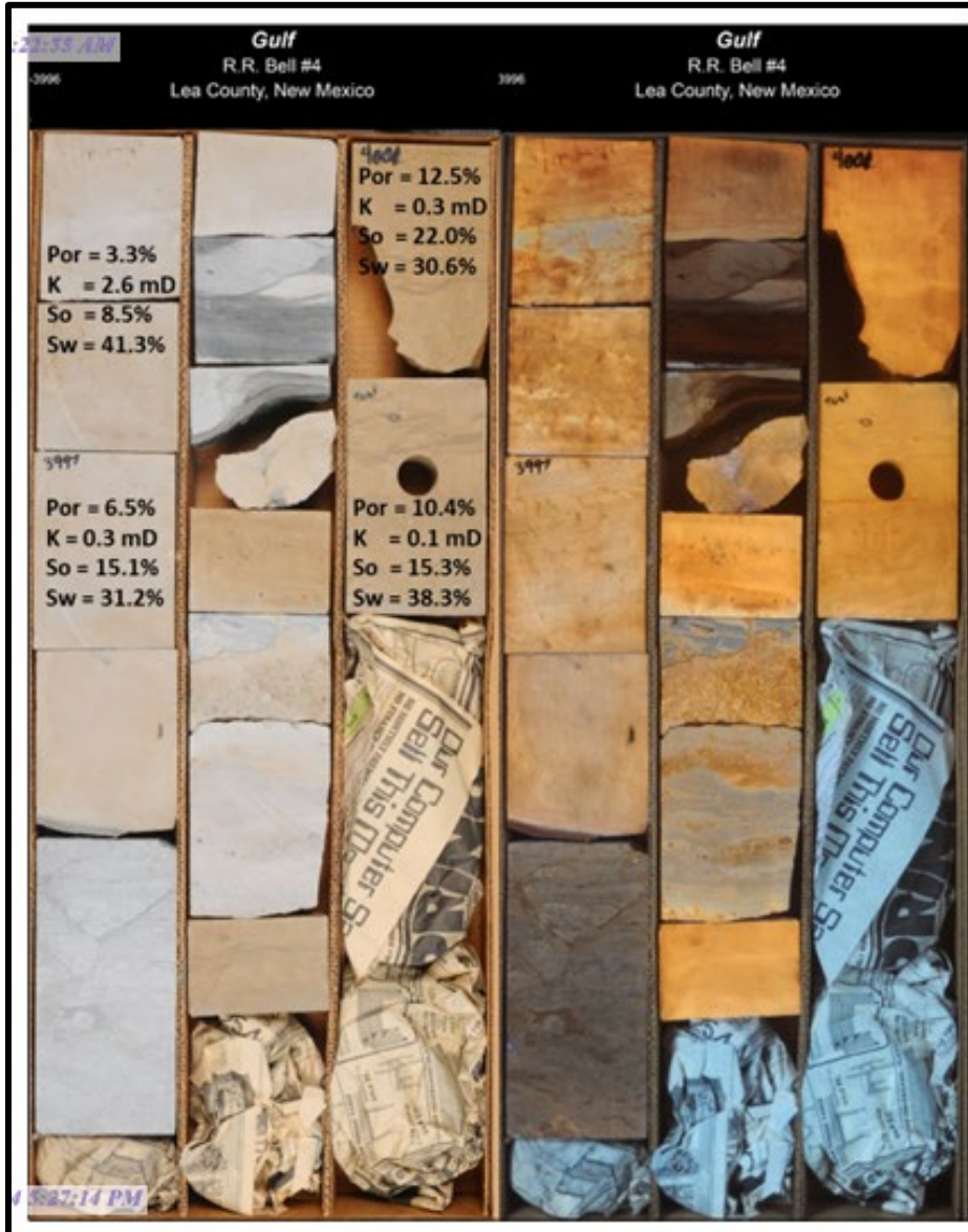
Exhibit L-11: One of the key indicators of an ROZ, the staining of the core with oil over the San Andres is strong evidence to the ROZ in the EMSU San Andres.
