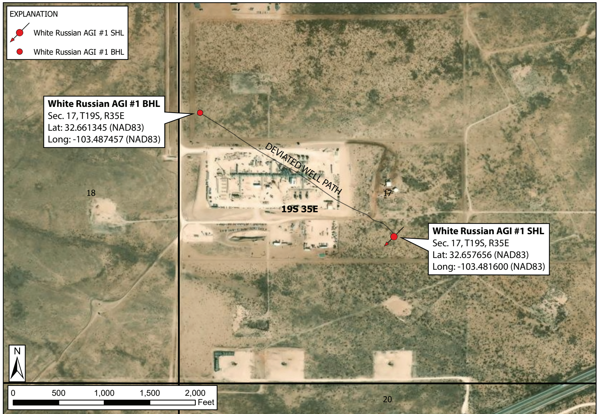
Figure 2. Aerial photographic location map showing the as-drilled White Russian AGI #1 well surface- and bottom-hole locations, and surface lands where the Dude Processing Plant has been constructed.
