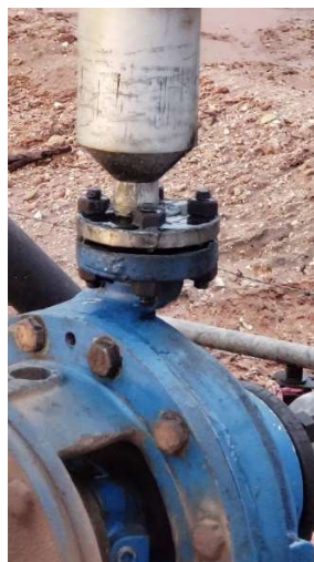
Broken Swedge at Pump source of Release
