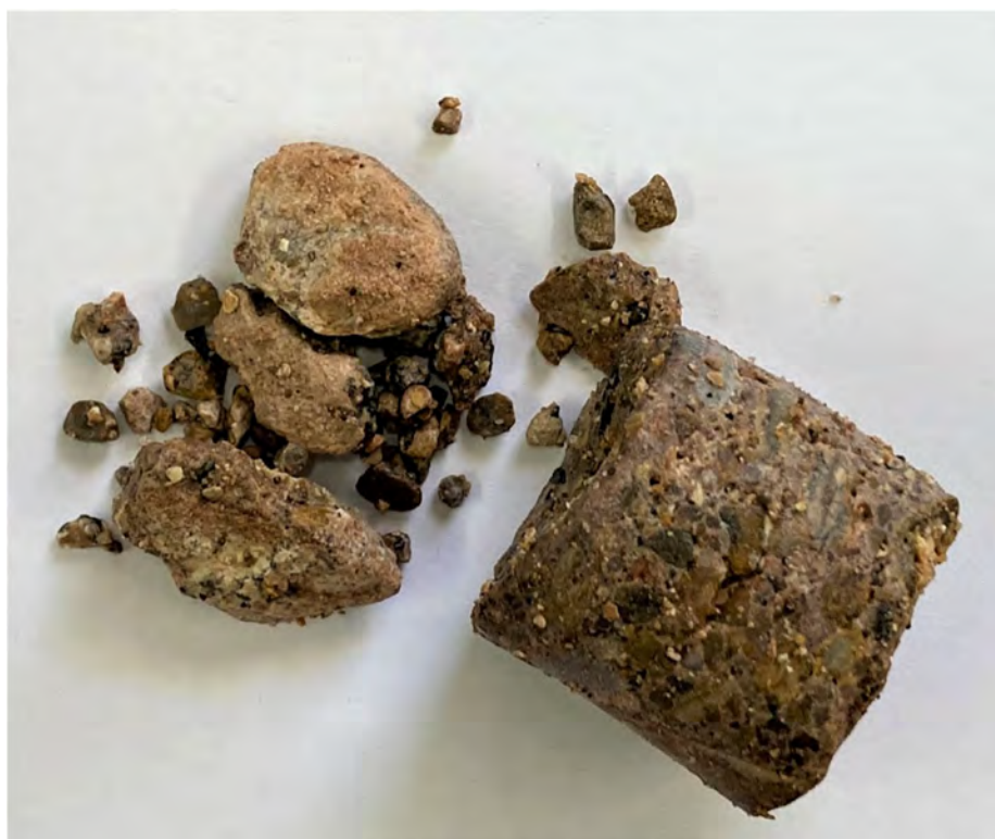
Photograph 2 – Small gravel with fine to coarse-grained sand conglomerate layer at approximately 5.5 feet bgs
