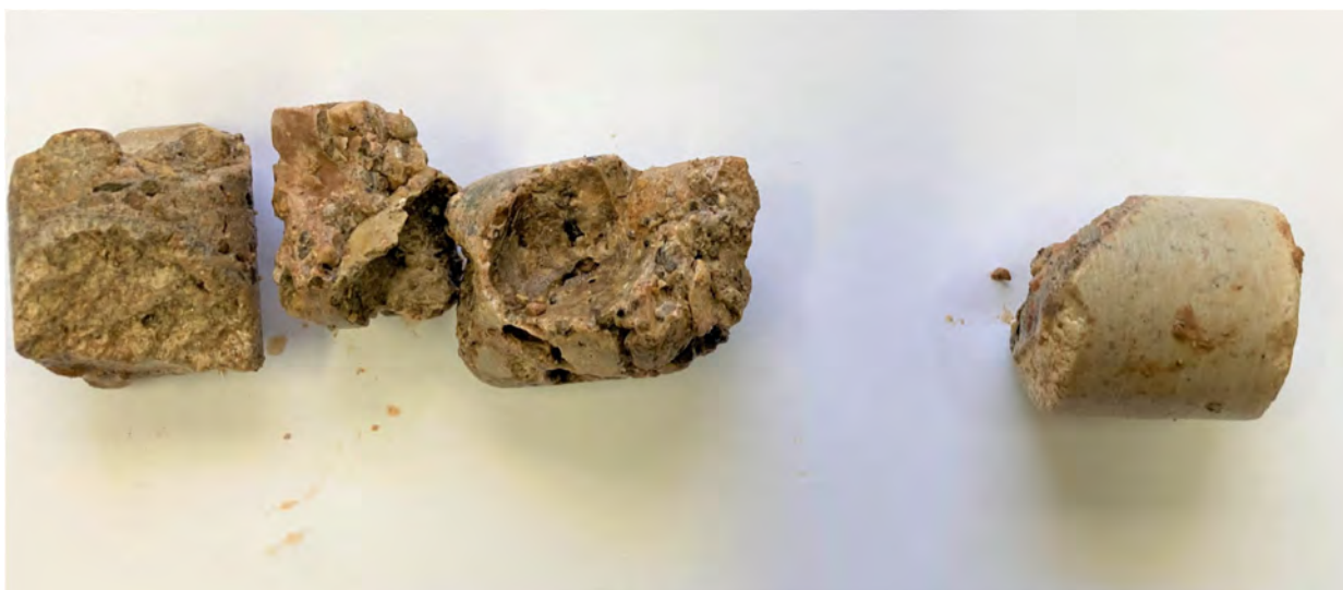
Photograph 4 – moderate to well-cemented small to large gravel conglomerate to full indurated caliche transition (from left to right)
