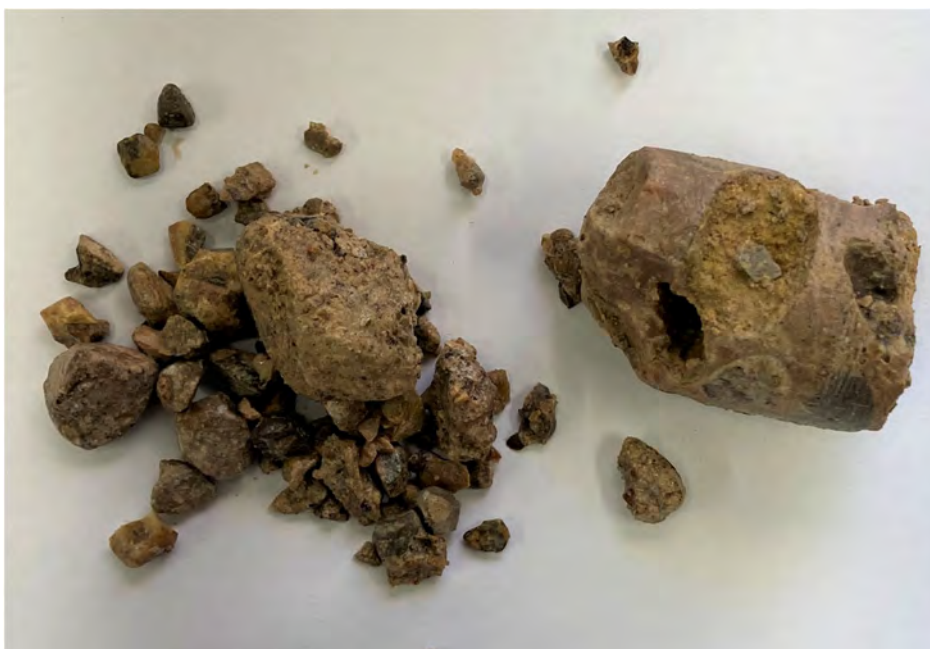
Photograph 3 –Moderately-cemented large gravel to indurated caliche transition
