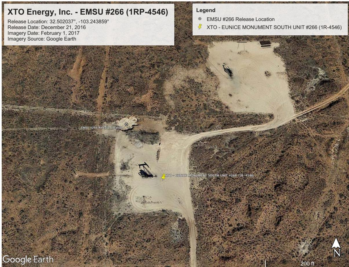
**Figure 4.** Georeferenced Google Earth Image Depicting Release Point Identified in the Initial C-141. The subject site is shown after the release at a period when remedial activities were likely performed to address the release. Note that an excavated area is visible at the release location.
