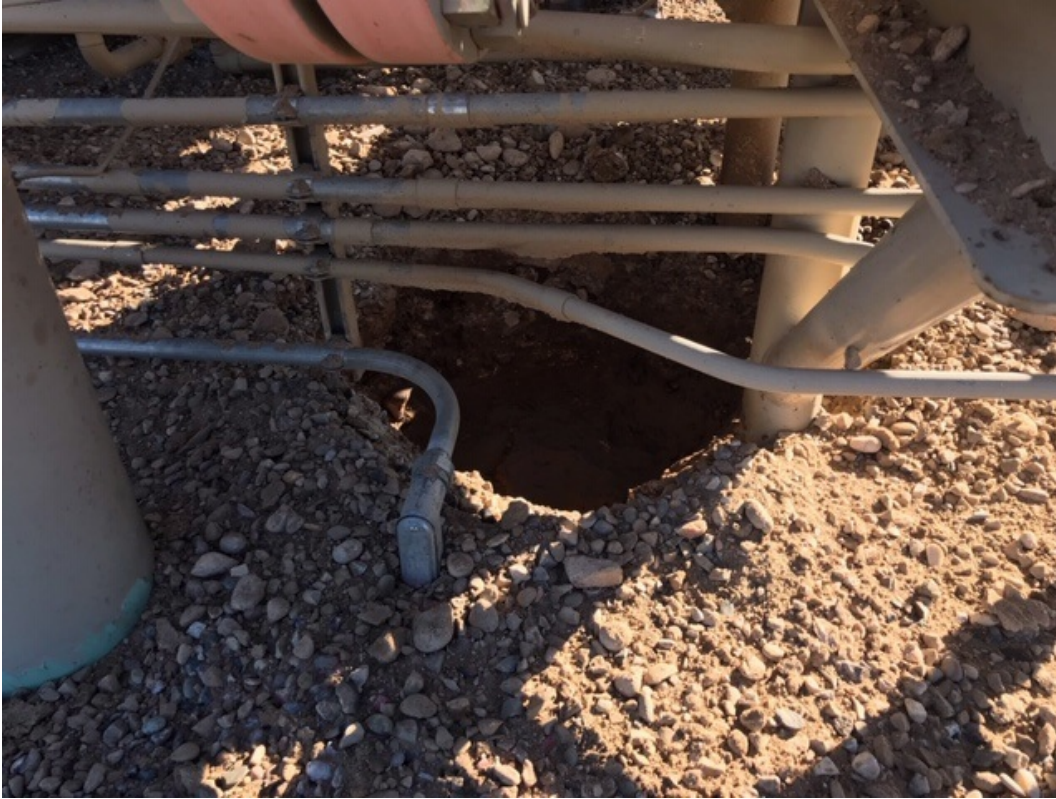
Photo 1: Hole created by released gas.
