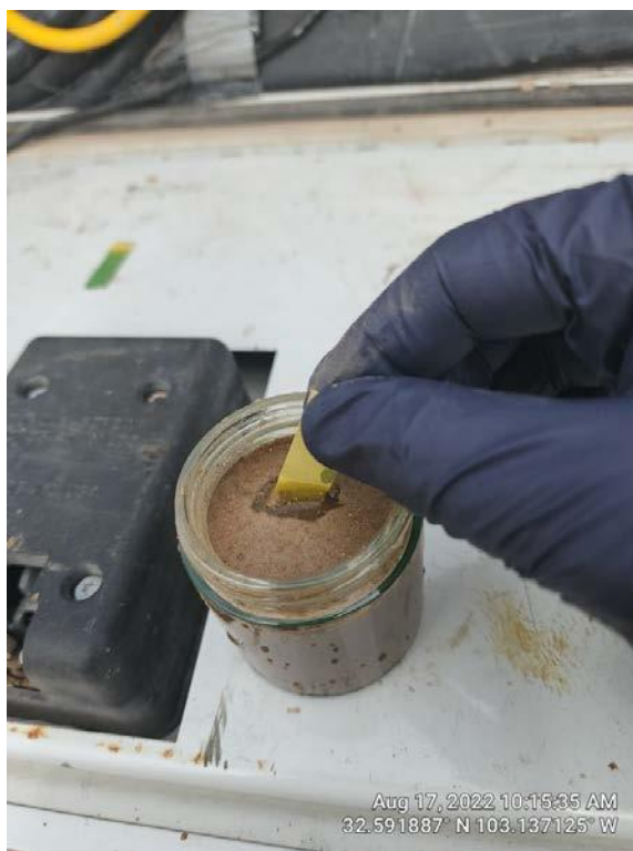
Figures 2 & 3 – Soil pH measurement from excavated material
