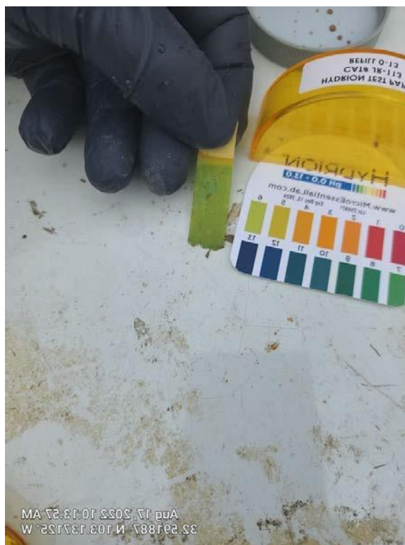
Figures 2 & 3 – Soil pH measurement from excavated material
