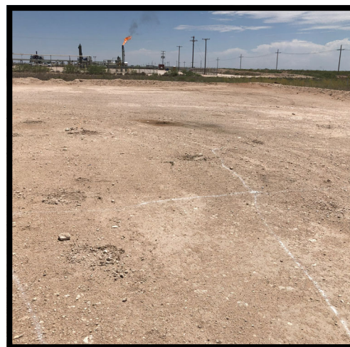
View of surficial soil confirmation sampling grid, facing south. Five point grab pattern visible.
