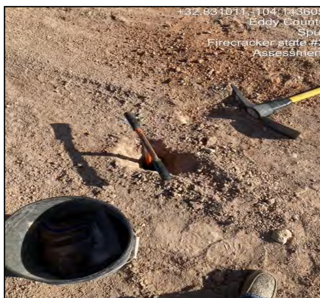
Photograph of hand auger going into the ground to collect samples.
