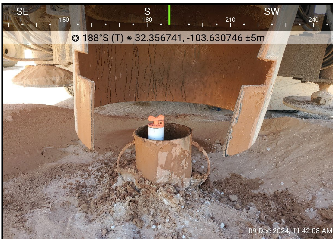
View of soil boring (C-4908-POD1) with temporary 2-inch pvc casing post drilling activities, facing south (December 9, 2024).
