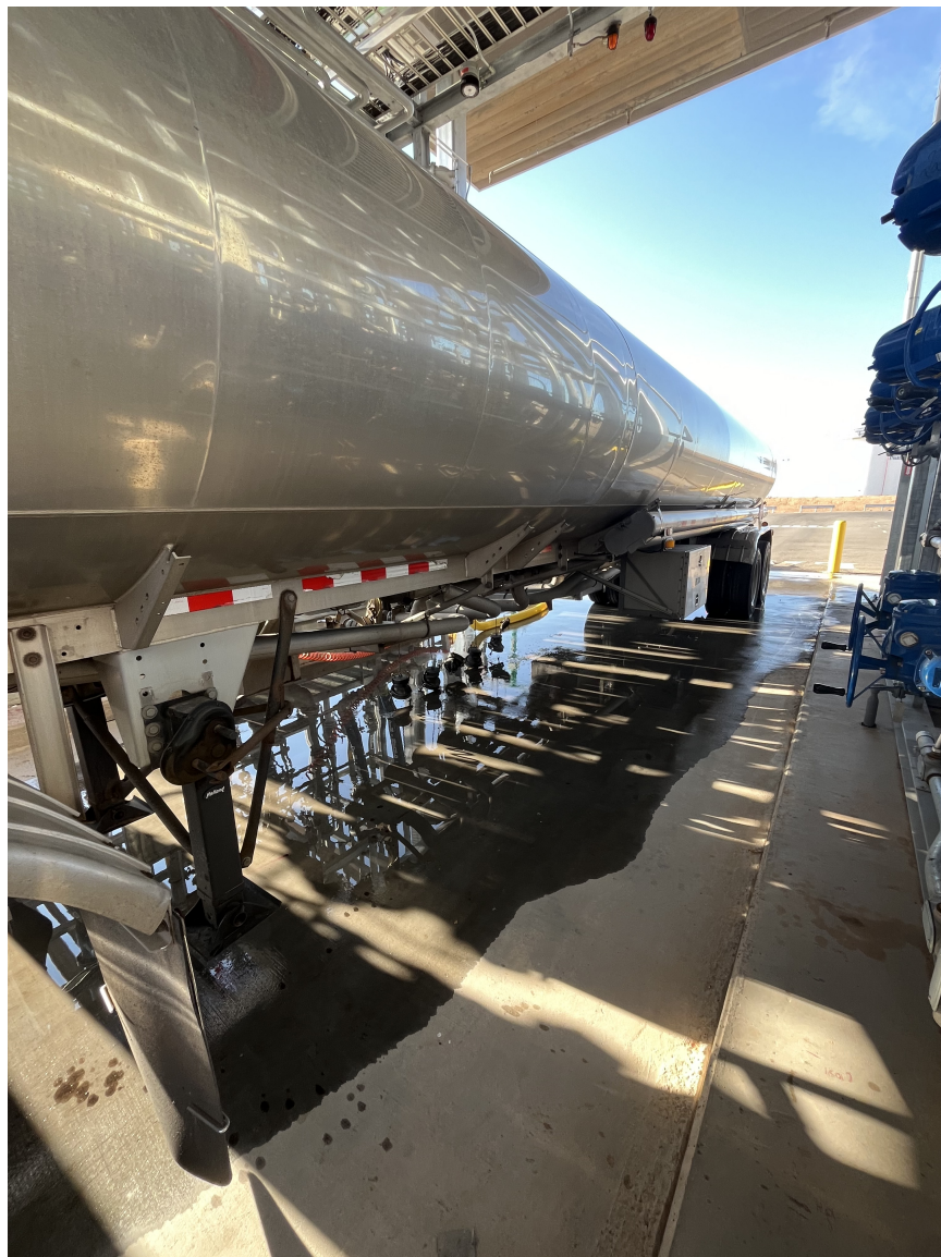
Photo 2: View for the diesel fuel overflowing from tanker truck.
