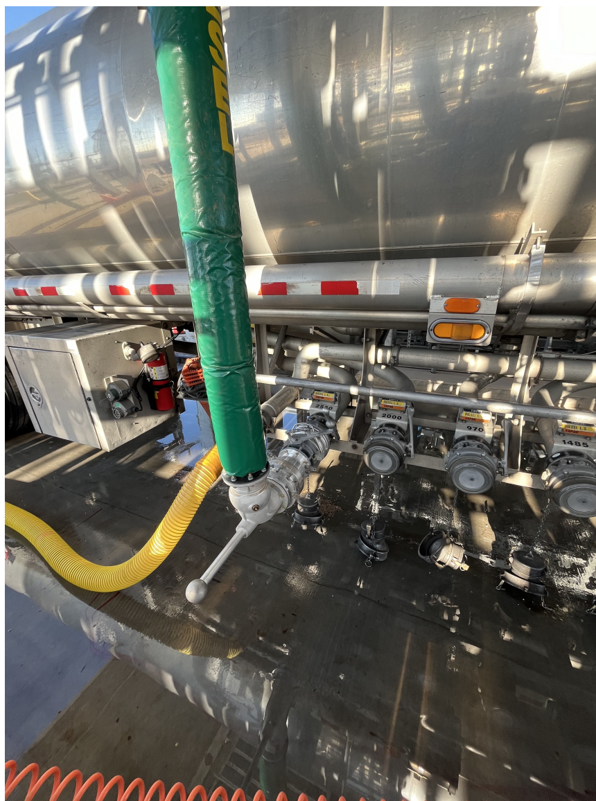
Photo 1: View for the diesel fuel overflowing from tanker truck.
