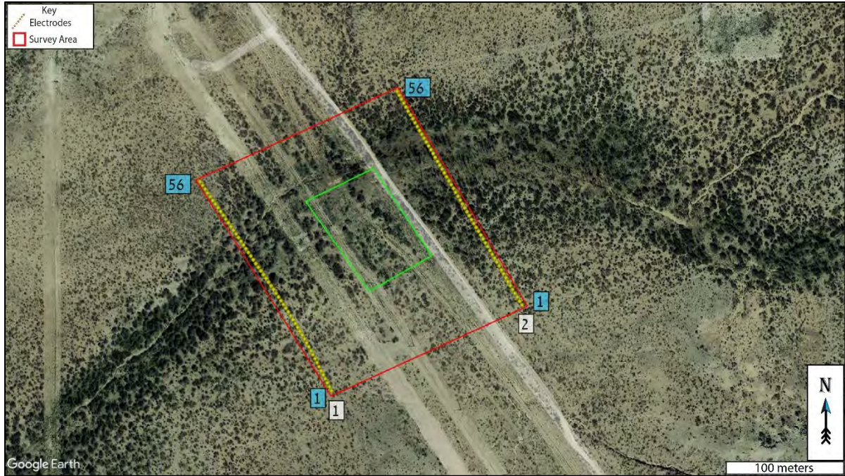
Figure 4: Survey overview. Two survey lines (denoted with white numbers) were conducted with 56 electrodes each at 4-meter spacing (yellow dots denoted with blue numbers). Background image credit: Google Earth. Image date: December 21, 2019. Image datum: WGS-84.
