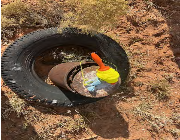
View of dry napkin out of hole after measuring to a depth of 105' bgs (12/5/24).
