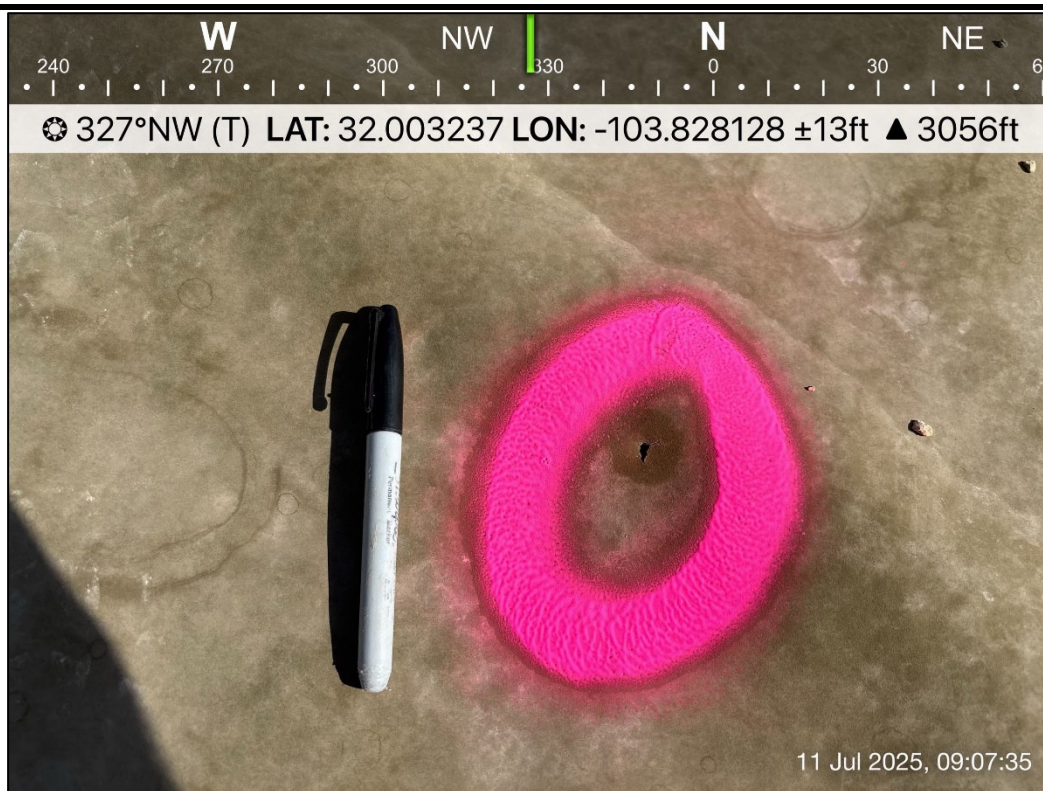
PHOTO 19: Northwestern view of failed liner integrity. 7/11/2025
