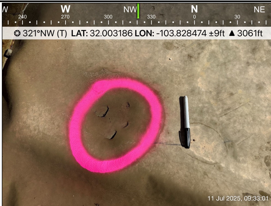
PHOTO 21: Northwestern view of failed liner integrity. 7/11/2025
